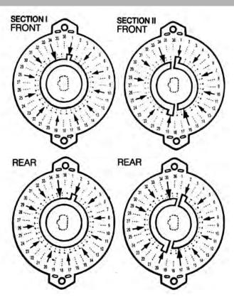
Switches with 12.85°, 25.7° & 18° angle of throw are available with higher lead time
