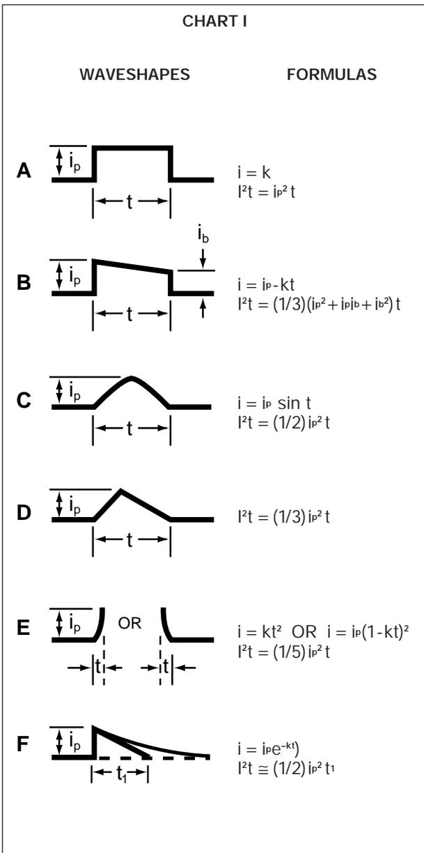
**Step 3** — Examine the  $I^2t$  rating data for the PICO® II, 125V, very fast-acting fuse. The part number 251001, 1 ampere design is rated at 0.256 A<sup>2</sup> Sec., which is the minimum fuse rating that will accommodate the 0.2327 A<sup>2</sup> Sec. value calculated in Step 2. This 1 ampere fuse will also accommodate the specified 0.75 ampere normal operating current, when a 25% derating factor is applied to the 1 ampere rating, as previously described.
